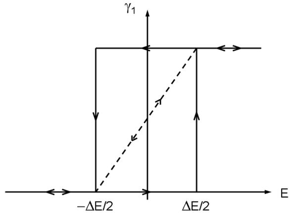
Fig. 1. Self-organized switching between two intersecting material flows on link 1 (permeability function  $\gamma_1(t) = 1$ ,  $\gamma_2(t) = 0$ ) and 2 ( $\gamma_1(t) = 0$ ,  $\gamma_2(t) = 1$ ) in dependence on the evolution of the quantity  $E(t)$  which balances the differences between the actual outflows  $\Delta O(t)$  and the total amounts of waiting material  $\Delta N(t)$  on each link.
