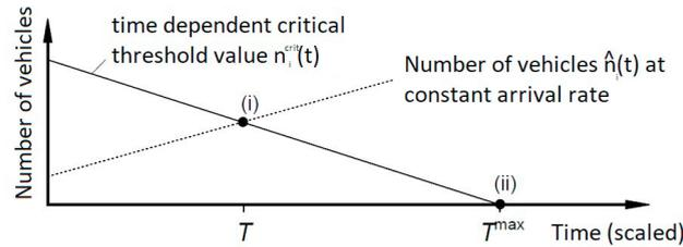
Fig. 1. Critical threshold value  $n^{crit}$  over time.<sup>2</sup>
